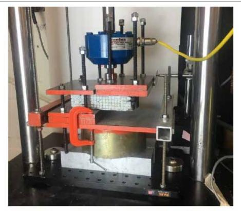
Figure 136. Finalized test setup for shear fatigue test
