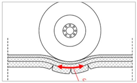
Schematic illustration of the deformation below the asphalt layer (source: *igbv*, *Lüneburg*)
